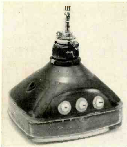
This view of the Colornetron beam-switching tube used in Japanese Yaou sets shows the three high-voltage electrode connections. The center pin is for the focusing grid, which gets 6.3 kv. The outer pins connect with the beam-switching grid, which gets 4.7 kv peak to peak.
